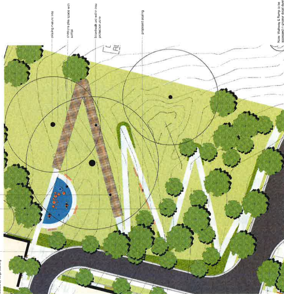
4 Pocket Park 4 - Accessible Path with Rest Points Detail Plan @ 1"=60'
